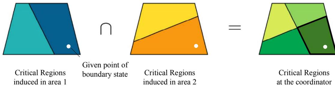
(a) Local parameterization: The bolded polytope is the critical region containing the given boundary state
